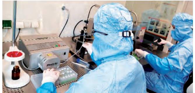
Filling vials with a peptide vaccine at the GMP Center in Tübingen (© Marion Richter / Immunology Dept.)
